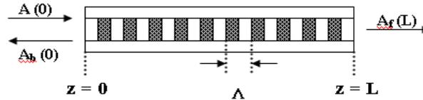
Figure 6: Schematic of a FBG of length  $L$  illuminated by electromagnetic field of amplitude  $A(z)$ .
