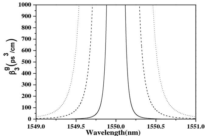
Figure 5: The third order dispersion parameter induced by FBG is plotted as a function of wavelength for three different values of the coupling coefficient  $\kappa = 10 \text{ cm}^{-1}$  (dotted curve),  $\kappa = 5 \text{ cm}^{-1}$  (dashed curve) and  $\kappa = 1 \text{ cm}^{-1}$  (solid curve).
