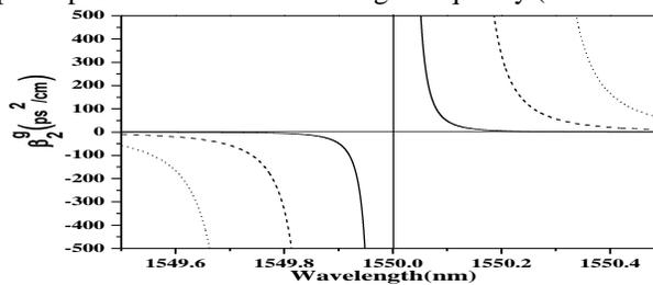
Figure 4: The second order dispersion parameter (GVD) of FBG is plotted as a function of incident wavelength for three different values of the coupling coefficient  $\kappa = 10 \text{ cm}^{-1}$  (dotted curve),  $\kappa = 5 \text{ cm}^{-1}$  (dashed curve) and  $\kappa = 1 \text{ cm}^{-1}$  (solid curve).
