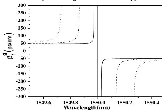
Figure 3: First order dispersion of FBG is plotted as a function of wavelength for three values of the coupling coefficient  $\kappa = 10 \text{ cm}^{-1}$  (dotted curve),  $\kappa = 5 \text{ cm}^{-1}$  (dashed curve) and  $\kappa = 1 \text{ cm}^{-1}$  (solid curve).
