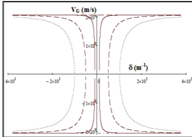
Figure 2: Curve showing variation of group velocity with in a fiber Bragg grating for three values of the coupling coefficient  $\kappa = 10 \text{ cm}^{-1}$  (dotted curve),  $\kappa = 5 \text{ cm}^{-1}$  (dashed curve) and  $\kappa = 1 \text{ cm}^{-1}$  (solid curve).
