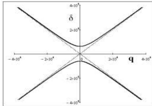
Figure 1: Dispersion curves showing variation of  $\delta$  with  $q$  and the existence of the photonic bandgap for a fiber grating.
