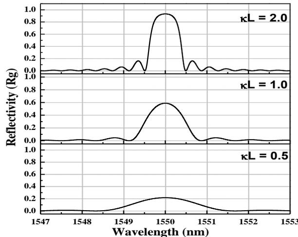
Figure 7: Calculated reflection spectral response as a function of wavelength for five different fiber Bragg gratings, with increasing lengths.
