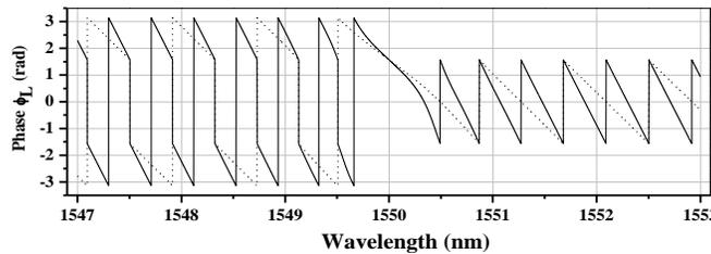
Figure 8: Variation in the phase ( $\phi_L$ ) of reflection coefficient ( $r_g$ ) plotted as a function of wavelength for two values of grating strength  $\kappa L = 1$  (dotted curve) and  $\kappa L = 2$  (solid curve).
